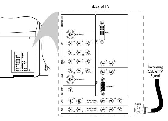
**NOTE:** This connection will supply stereo sound to the TV if it is being broadcast by the station you are watching.
